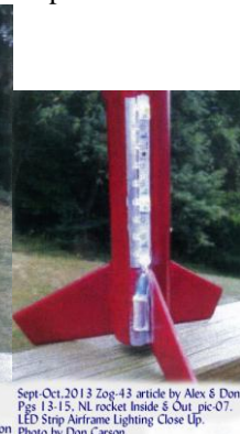
Sept-Oct.2013 Zog-43 article by Alex & Don: Pgs 13-15: NL rocket Inside & Out, pic-06: LED Strip Airframe Lighting. Photo by Don Carson
