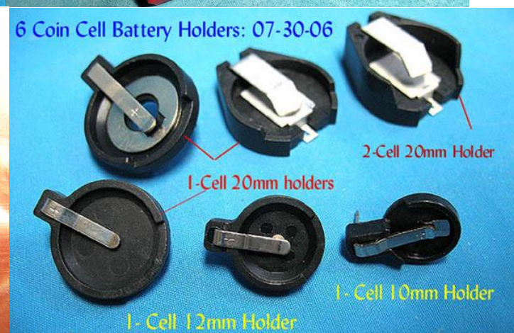
3 volt Lithium Coin Cells CR-2032 (20mm), BR-1225 (12.5mm) & CR-1025 (10 MM)
