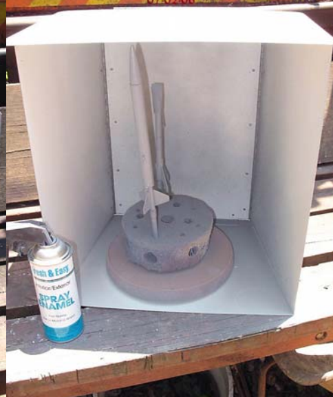
All Aluminum, portable. Store & Use Outdoor Micro Spary Booth. "Answer to the Cardboard box:D" First Use. Priming two micro models. Top closed 07-02-06
