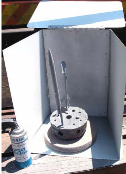
All Aluminum, portable. Store & Use Outdoor Micro Spary Booth. "Answer to the Cardboard box:D" First Use. Priming two micro models. 07-02-06
