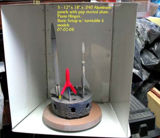
All Aluminum, portable. Store & Use Outdoor Micro Spary Booth. "Answer to the Cardboard box:D" First Use. Priming two micro models. Top closed 07-02-06
