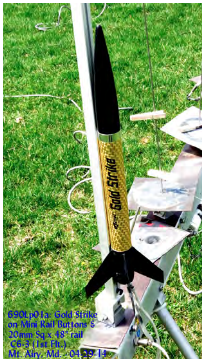
Rail used to replace an 1/8" launch rod Photo: J. McCoy
