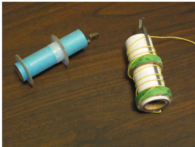
Original and upgraded motor mounts. Note the heaved up centering rings and Kevlar shock cord mount. I ground the top end of the retaining hook down flush with the inside surface of the motor block to ensure a correct fit for single use composites, although in this case their use is highly unlikely.
