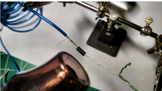
Fig. 7: Heat shrink the core solder joint.
