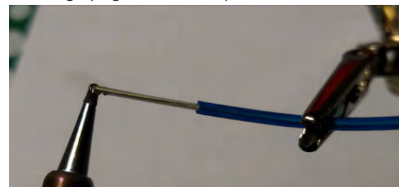
Fig. 3: Burning off the PVC coating.
