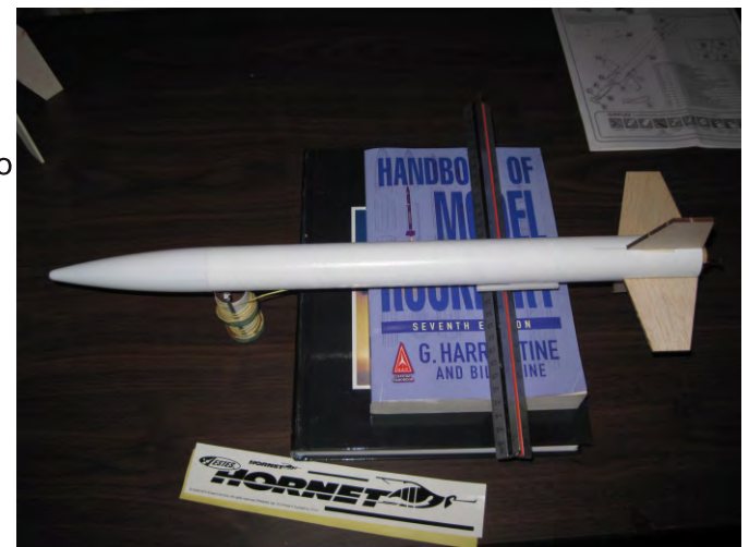
Balancing a pre-assembled model (suspending by a string would work as well). This model was pre-assembled exactly per manufacturer's instructions with parachute, shock cord, and recovery wadding inside, and a C6-5 motor installed in the original motor mount. The fins are held on with double sided tape. The balance point locates the mass center appropriate for stable flight.
