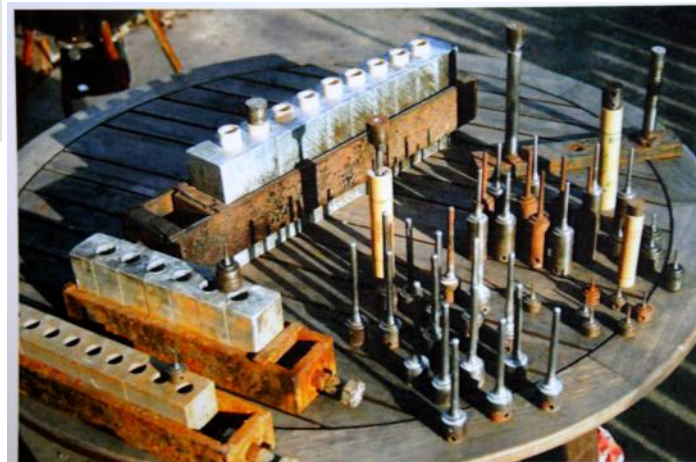
This equipment is for the manufacture of handmade black powder rocket motors. The long mandrels are for making high thrust, short duration motors to lift heavier loads. The short mandrels with the narrow throat diameters are for making long duration, end-grain burning motors capable of sending rockets with light payloads to higher altitudes. Multi-staging is also common.
