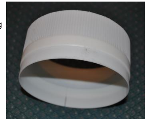
3D printed corrugated tube.
