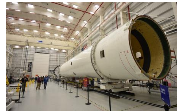
A wide view inside the Horizontal Integration Facility looking down the 90.9 feet length of the Antares first stage.
